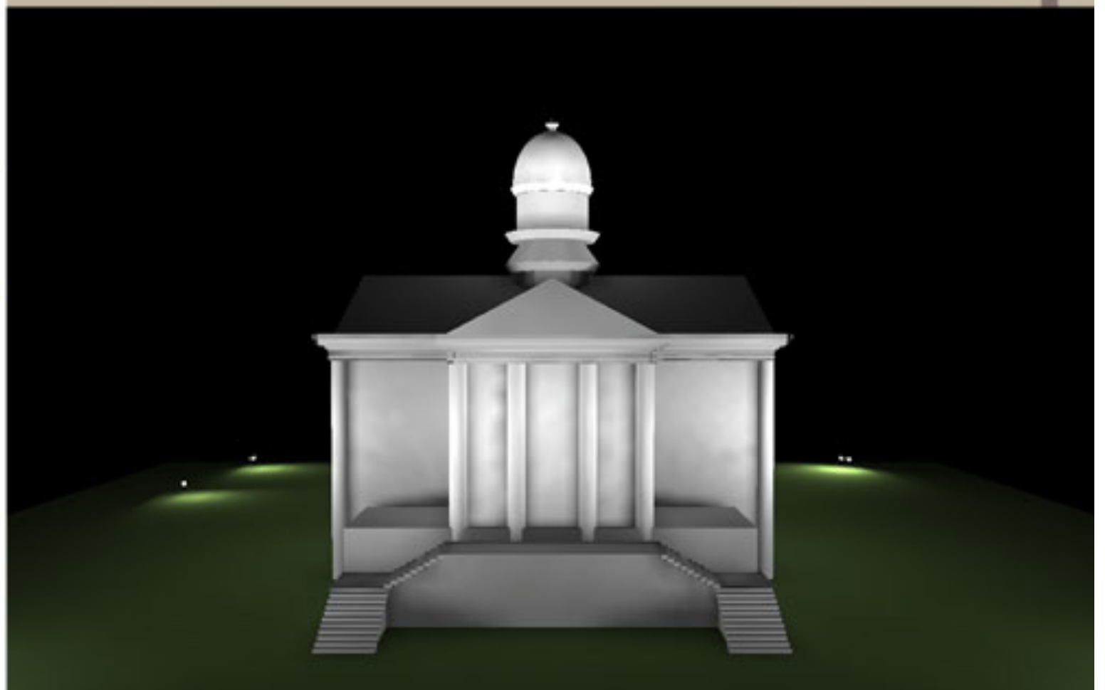
Top-Left: The courthouse floodlighting was extremely limited in terms of possible locations. This illustration shows both the model and the calculation points. Bottom-Right: The front facade was the most critical area in regards to lighting levels. This design does not account for decorative poles along the entry walkway.
